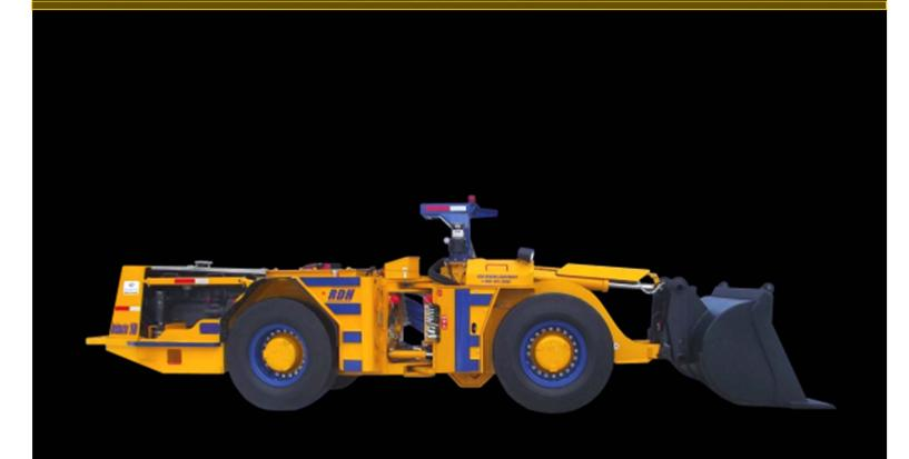
Bucket capacities between 1.5 m³ to 2.3 m³
