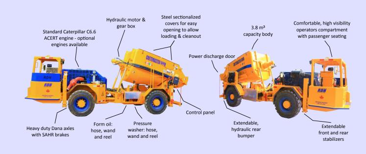
The robust and reliable four-wheel drive, articulated Cretemaster 600R-TL consists of a power-shift transmission powered by a choice of diesel engines connected to heavy-duty Dana axles. The rugged frame and articulated carrier make the Cretemaster 600R-TL a very durable and extremely maneuverable unit even in the tightest situations. Incorporating a full sweep agitator-remixer the Cretemaster 600R-TL provides a faster, safer, more efficient means of placing concrete.
