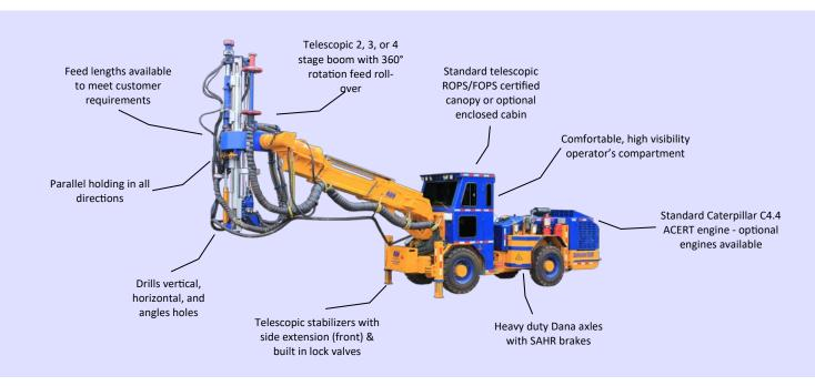
The productive, safe, and reliable Boltmaster 150 is a fully mechanized rock bolting rig designed for underground mining and tunneling operations. The robust and reliable four-wheel drive, articulated Boltmaster 150 consists of a power-shift transmission powered by a choice of diesel engines connected to heavy-duty Dana axles. The rugged frame and articulated carrier make the Boltmaster 150 a very durable and extremely maneuverable unit even in the tightest situations.
