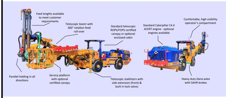
The productive, safe, and reliable Boltmaster 200 is a fully mechanized rock bolting rig designed for underground mining and tunneling operations. The robust and reliable four-wheel drive, articulated Boltmaster 200 consists of a power-shift transmission powered by a choice of diesel engines connected to heavy-duty Dana axles. The rugged frame and articulated carrier make the Boltmaster 200 a very durable and extremely maneuverable unit even in the tightest situations.
