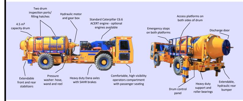
The robust and reliable four-wheel drive, articulated Cretemaster 600R consists of a power-shift transmission powered by a choice of diesel engines connected to heavy-duty Dana axles. The rugged frame and articulated carrier make the Cretemaster 600R a very durable and extremely maneuverable unit even in the tightest situations. Incorporating an efficient and reliable concrete remixer system, the Cretemaster 600R provides a faster, safer, more efficient means of placing concrete.
