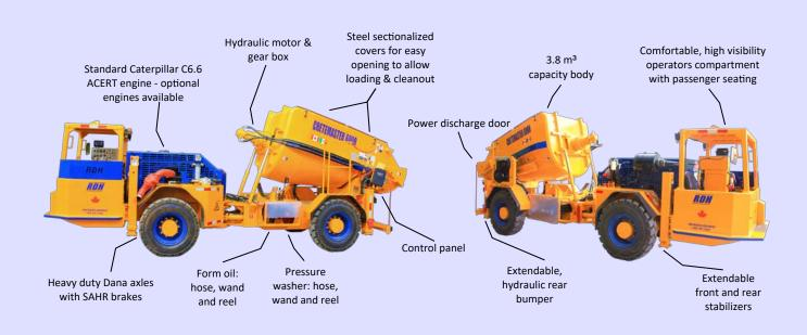
The robust and reliable four-wheel drive, articulated Cretemaster 600R-TL consists of a power-shift transmission powered by a choice of diesel engines connected to heavy-duty Dana axles. The rugged frame and articulated carrier make the Cretemaster 600R-TL a very durable and extremely maneuverable unit even in the tightest situations. Incorporating a full sweep agitator-remixer the Cretemaster 600R-TL provides a faster, safer, more efficient means of placing concrete.
