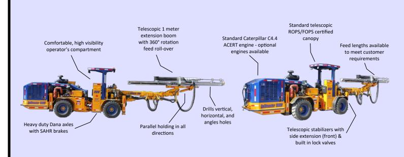
The productive, safe, and reliable Drillmaster 100 is designed face drilling in underground narrow vein mining and tunneling operations. The robust and reliable four-wheel drive, articulated Drillmaster 100 consists of a power-shift transmission powered by a choice of diesel engines connected to heavy-duty Dana axles. The rugged frame and articulated carrier make the Drillmaster 100 a very durable and extremely maneuverable unit even in the tightest situations.
