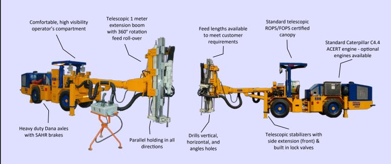
The productive, safe, and reliable Drillmaster 100 Longhole is designed for longhole drilling in underground mining and tunneling operations. The robust and reliable four-wheel drive, articulated Drillmaster 100 Longhole consists of a power-shift transmission powered by a choice of diesel engines connected to heavy-duty Dana axles. The rugged frame and articulated carrier make the Drillmaster 100 Longhole a very durable and extremely maneuverable unit even in the tightest situations.
