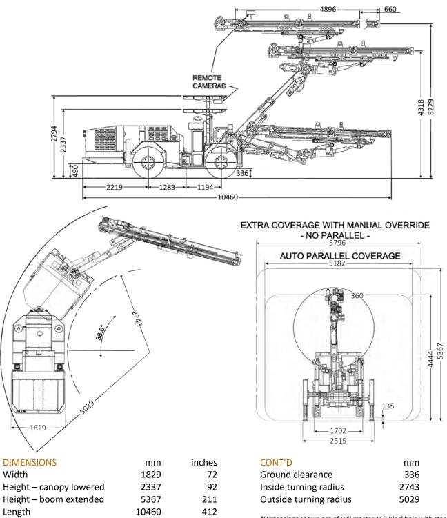
\*Dimensions shown are of Drillmaster 150 Blockhole with standard options, a 2 stage boom and 10.00 x 20 tires. Alternate configurations may affect dimensions.
