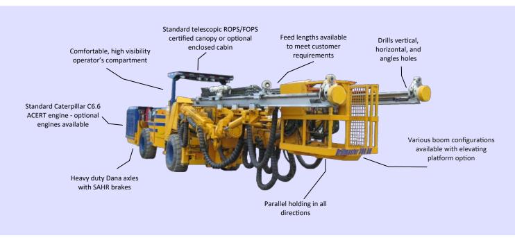
The productive, safe, and reliable Drillmaster 300 is designed for face drilling in underground mining and tunneling operations. The robust and reliable four-wheel drive, articulated Drillmaster 300 consists of a power-shift transmission powered by a choice of diesel engines connected to heavy-duty Dana axles. The rugged frame and articulated carrier make the Drillmaster 300 a very durable and extremely maneuverable unit even in the tightest situations.
